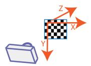
When you reconstruct a 3-D scene from multiple views containing a calibration pattern, the resulting 3-D points are defined in the pattern-based coordinate system. The "Sparse 3-D Reconstruction From Two Views" example shows how to reconstruct a 3-D scene from a pair of 2-D images containing a checkerboard pattern.
