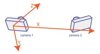
When you reconstruct a 3-D scene using a calibrated stereo camera, the reconstructScene and triangulate functions return 3-D points with the origin at the optical center of Camera 1. When you use Kinect® images, the depthToPointCloud function returns 3-D points with the origin at the center of the RGB camera.
